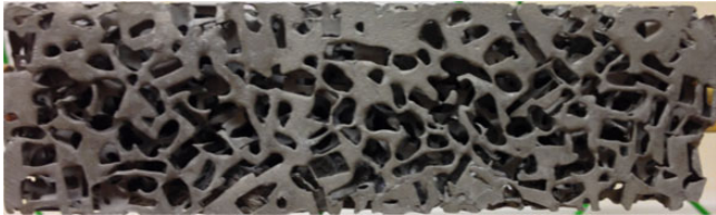
Figure 14. A metal foam that is used to enhance PCM performance.
