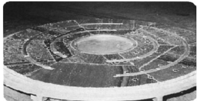
Figure 17. A porous honeycomb structure with circumferential heat pipes for isothermalization [17]. Reprinted from Reay and Harvey [17]. The role of heat pipes in intensified unit operations, pp. 147–153, 2013 with permission from Elsevier.
