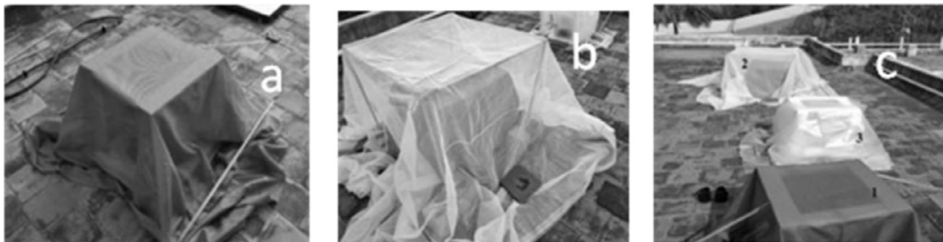
Fig. 1: Three housing systems (a) Single shade-net, (b) double shade-net, and (c) Polythene sheet housing
