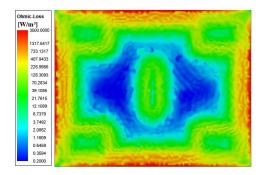
Figure 10. Loss distribution diagram of the aluminum plate in simulation results.
