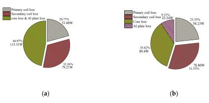
Figure 20. Loss ratio of simulation and experiment. (a) Loss ratio of the experiment; (b) loss ratio of simulation.
