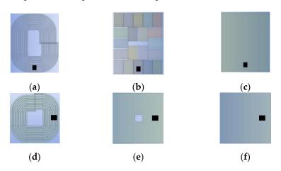
**Figure 21.** Embedded position of thermocouple sensors. (a) Primary coil; (b) primary magnetic core; (c) primary aluminum plate; (d) secondary coil; (e) secondary magnetic core; and (f) secondary aluminum plate.
