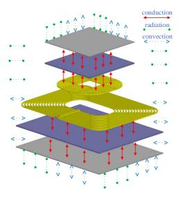
Figure 13. Schematic diagram of heat transfer mode of the magnetic coupler.
