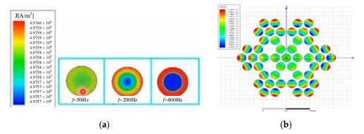
**Figure 2.** Schematic diagram of solid copper wire's skin effect and proximity effect. (**a**) Skin effect; (**b**) proximity effect.
