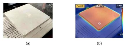
**Figure 24.** The temperature of secondary shielding aluminum plate coated with thermal conductive silicone grease. (a) Shielding aluminum plate coated with thermal conductive silicone grease; (b) temperature value and distribution.
