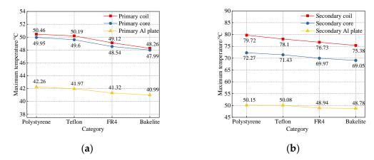
**Figure 17.** Variation of the maximum temperature of each part of the magnetic coupler with supporting material. (a) Primary magnetic coupler; (b) secondary magnetic coupler.
