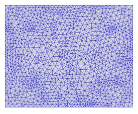
Figure 11. Grid division of aluminum plate.
