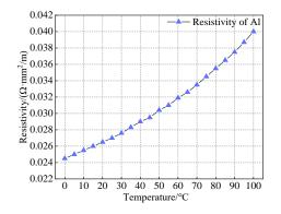
Figure 12. Variation curve of aluminum resistivity with temperature.
