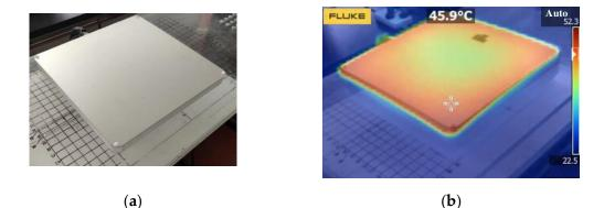
**Figure 22.** The temperature of the secondary shielding aluminum plate of the magnetic coupler. (**a**) The shielding aluminum plate; (**b**) the temperature value and distribution of the shielding aluminum plate.
