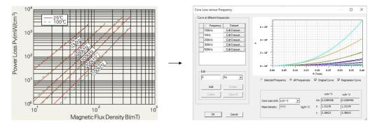
Figure 6. B-P curve data fitting of magnetic ferrite core.
