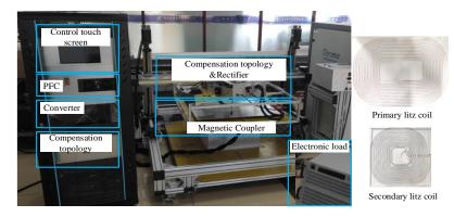
Figure 19. A 6.6 kw electric vehicle wireless charging system experimental platform.
