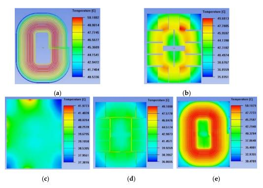
**Figure 14.** The temperature of each part of the primary magnetic coupler. (**a**) Primary coil; (**b**) primary magnetic core; (**c**) primary aluminum plate; (**d**) primary cover plate; and (**e**) primary wire tray.
