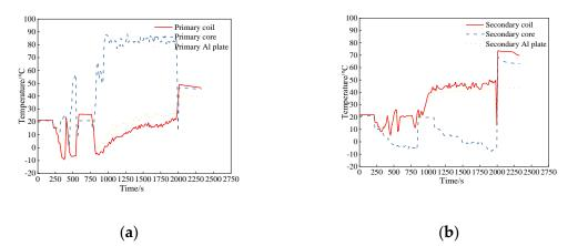
**Figure 23.** Temperature curve of each part of the magnetic coupler. (**a**) Temperature curve of each part of the primary side; (**b**) temperature curve of each part of the secondary side.
