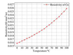
Figure 4. Change curve of copper resistivity with temperature.
