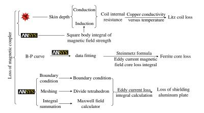
Figure 1. Loss calculation formula of each part in the magnetic coupler.
