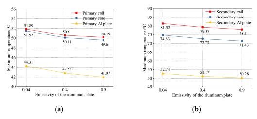
**Figure 18.** Variation of the maximum temperature of each part of the magnetic coupler with emissivity of the aluminum plate. (a) Primary magnetic coupler; (b) secondary magnetic coupler.
