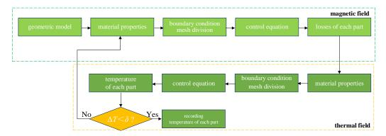
Figure 16. The magnetic coupler's thermal design steps.
