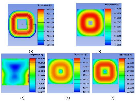
Figure 15. The temperature of each part of the secondary magnetic coupler. (a) Secondary coil; (b) secondary magnetic core; (c) secondary aluminum plate; (d) secondary cover plate; and (e) secondary wire tray.
