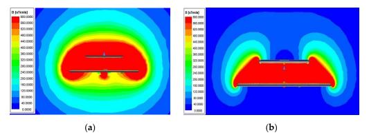
**Figure 7.** Cloud diagram of the magnetic induction intensity distribution in the magnetic coupler under different conditions. (a) Magnetic induction intensity distribution without aluminum plate; (b) magnetic induction intensity distribution with aluminum plate.
