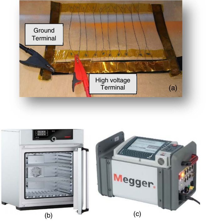
Fig. 1. Measurement Setup (a) Specimen's Holder in an unaged condition (b) MEMMERT UF260 Oven (c) Diagnostic Device MEGGER 4000
