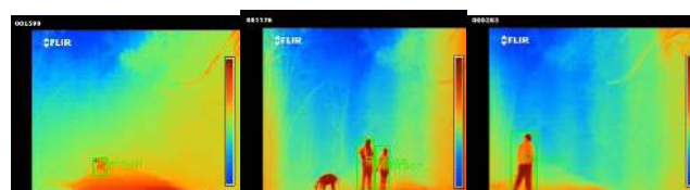
FIGURE 22. Results of person detection on images recorded with a normal lens in foggy weather: crouched walk, 50 m (left), standing still, <30 m (middle), normal walk, <30m (right).
