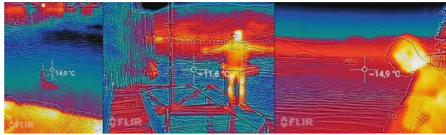
FIGURE 4. IR sensors are very sensitive to changes in ambient temperature.
