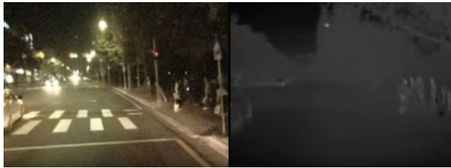
FIGURE 1. Night vision (left) vs. thermal imaging (right) [20].
