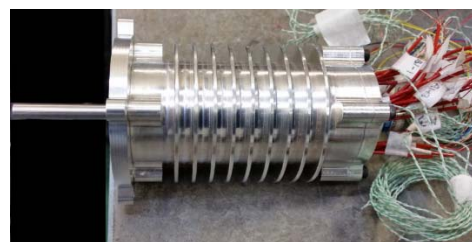
Fig. 3. PMSM driving the landing gear EMA.
