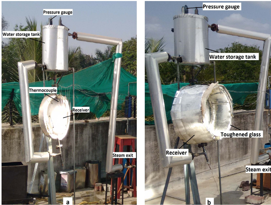
Figure 1. Photograph of (a) Unglazed receiver (b) Glazed receiver
