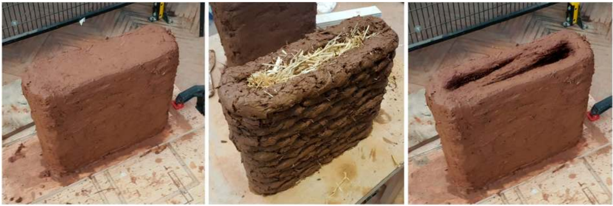
Figure 5. Samples of the 3d printed cob. From left to right; solid, single gap with straw filling and double gap.
