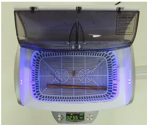
Figure 3. Cleaning the parts of the thermosyphon in the ultrasonic bath.
