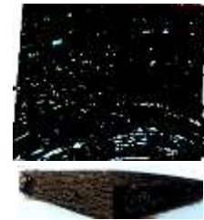
Fig. 3b: Specimen after TGA Test
