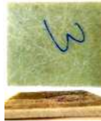
Fig. 3a: Specimen before TGA Test
