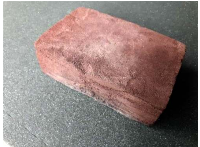
FIGURE 9 Demonstrator brick of JSC-2A sintered under ambient conditions. JSC, Johnson Space Center
