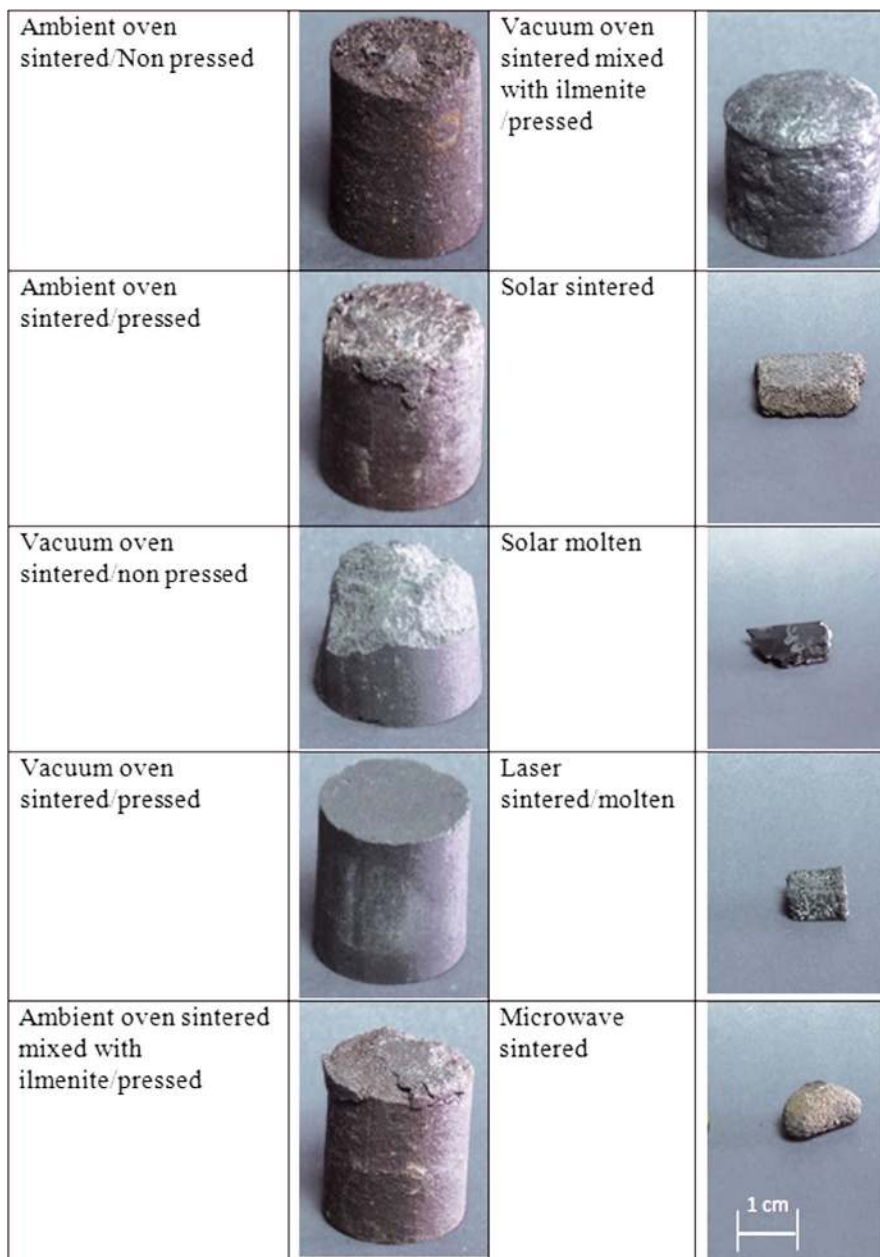
FIGURE 3 Fabricated parts using different strategies mentioned in methodology section, the scale bar applies for all the fabricated samples
