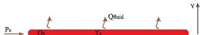
FIG. 2. Schematic of heat balance in a TA sound source. Part of input energy is consumed in TA sound source and the rest is conducted to the surrounding medium.
