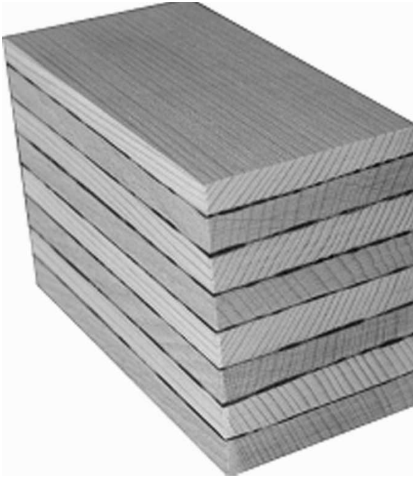
Figure 10. A wooden multi-layer element made of alternate layers of spruce and beech bonded by circular friction welding (Stamm 2005)
