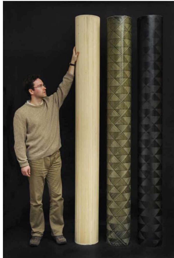
Figure 13. Wood tube of densified spruce (left) and filament winding of moulded tubes (right)
