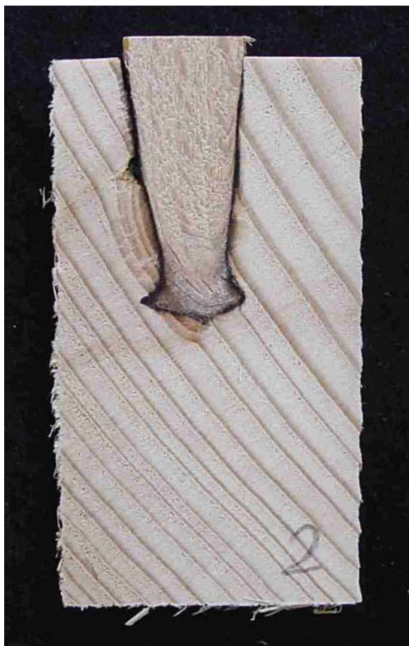
Figure 8. Cross-sectional profile of a dowel ligno-bonded by rotary friction welding (Ganne-Chédeville et al. 2005)
