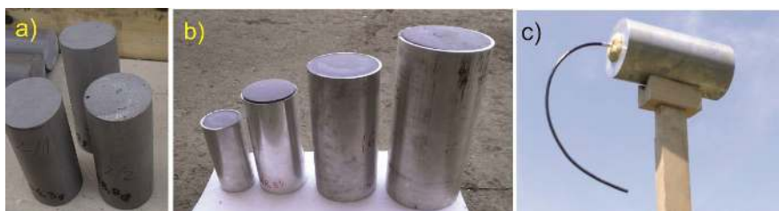
Figure 1. The explosive charges of different calibres (a,b) and the experimental model placed on a stand (c).
