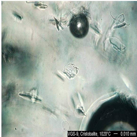
Figure 3. Crystals of Cristobalite in Low-Al 2 O 3 -Low-CaO Glass, 1020°C
