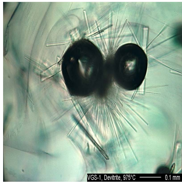
Figure 10. Crystals of Wollastonite and Probably Devitrite, Nucleated on a Bubble, in High- \text{Al}_2\text{O}_3 -Baseline Glass, 975°C
