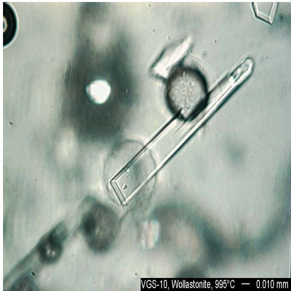
Figure 7. Crystals of Wollastonite in Low- \text{Al}_2\text{O}_3 -High-CaO Glass, 995°C
