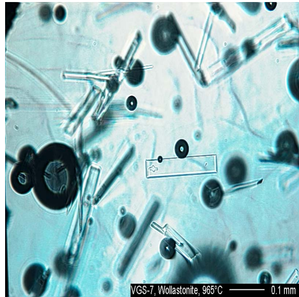
Figure 8. Crystals of Wollastonite in High- \text{Al}_2\text{O}_3 -High- \text{Na}_2\text{O} Glass, 965°C
