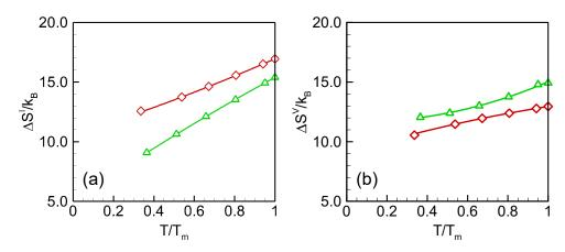
**Figure 4.** Formation entropies of (**a**) self-interstitial and (**b**) vacancy in germanium crystal. Red and green are results of SW and Tersoff, respectively. The lines are quadratic-fitted.
