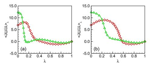
**Figure 2.** The integrands at different  $\lambda$  for (**a**) self-interstitial and (**b**) vacancy. Red for SW and green for Tersoff. The lines are guides for eyes.
