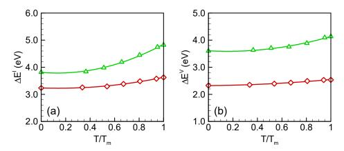
**Figure 1.** Formation energies of (**a**) self-interstitial (**b**) vacancy in germanium crystal. Red diamond and green delta symbols represent SW and Tersoff potential results, respectively. The lines are quadratic-fitted.
