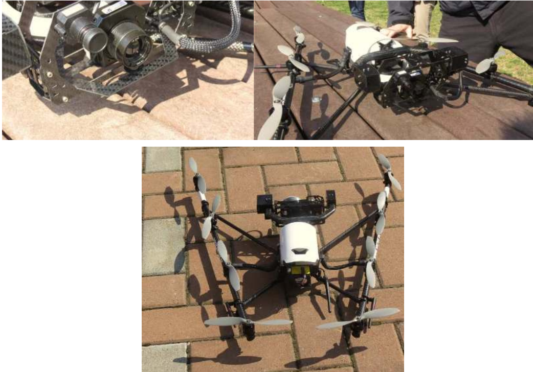
Figure 2 The ASCTEC Falcon 8 equipped with a FLIR Tau 640 thermal camera.
