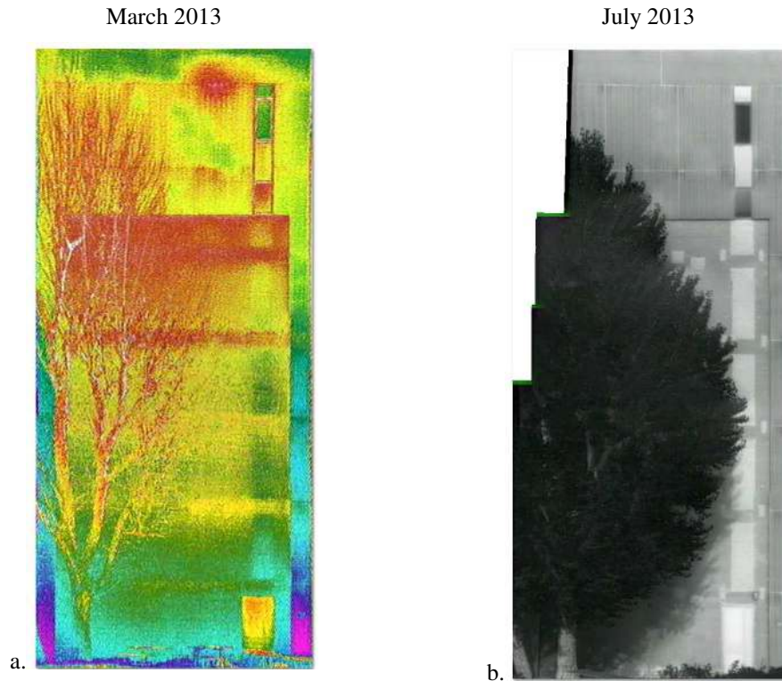
Figure 12 Facade thermal orthophoto: March 2013 (a), July 2013 (b).
