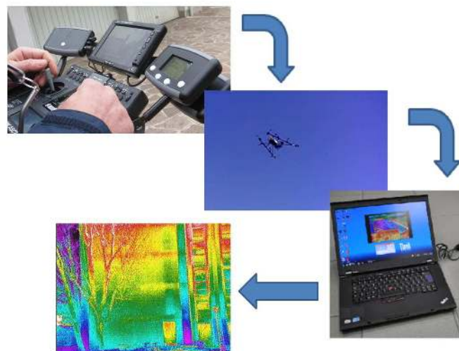
Figure 3 The thermal image acquisition procedure with the Falcon 8 system.
