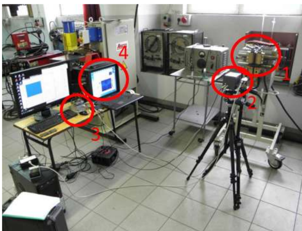
Fig. 6 Laboratory test bench. 1-heating source, 2-infrared camera, 3-thermocouple transmitter and ADC converter, 4-PC
