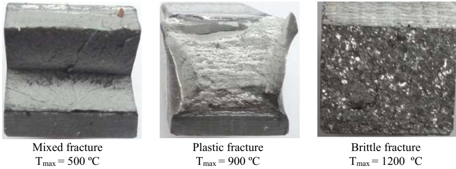
Fig. 20 View of S700MC steel HAZ fracture after an impact test at -30\text{ }^{\circ}\text{C}
