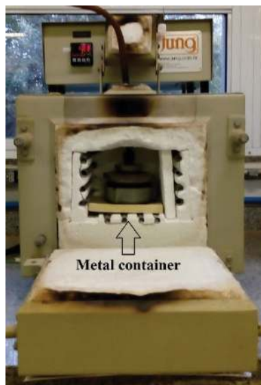
Figure 1. Experimental assembly for charcoal production
