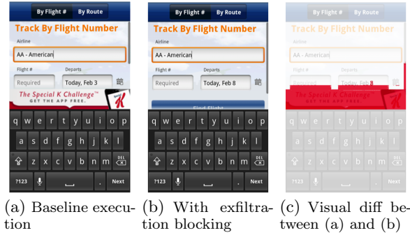
Figure 3: Detecting side effects using visual diff: The red shaded region in (c) highlights the advertising banner missing from (b).
