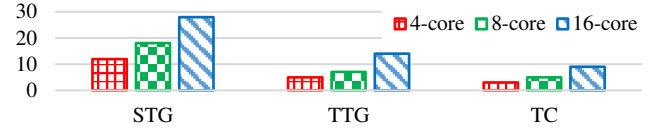
Fig. 10 Number of thermal violations occurred in one run of blackscholes benchmark for different number of cores when no thermal stress-aware approach applied
