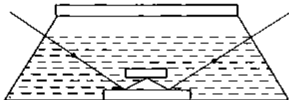
FIGURE 1. Schematic drawing of adsorption cell showing two chrome slides arranged for triple reflection of the polarized light beam.
