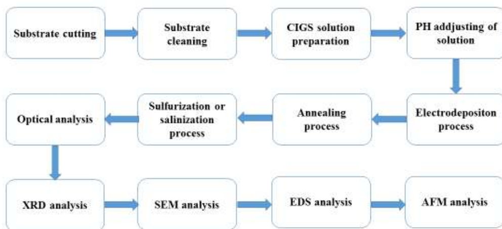
Figure 3.1 A flowchart of the process used for depositing all samples on different substrates.
