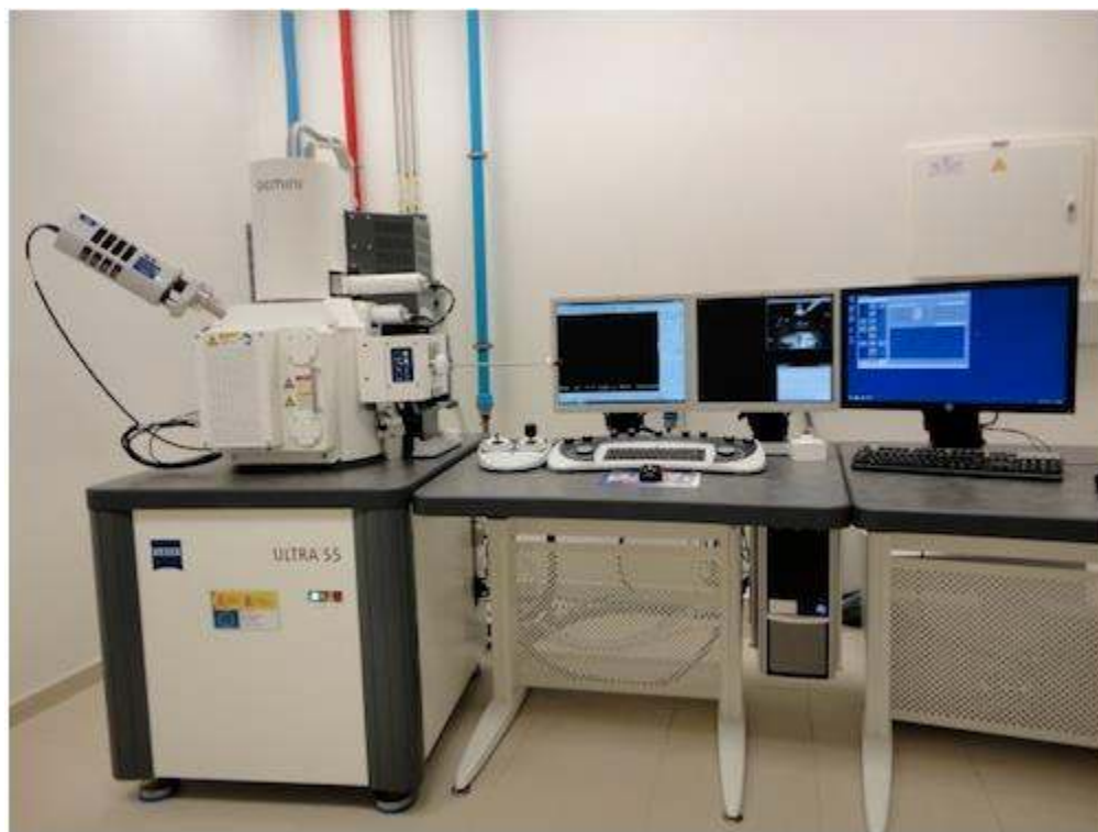
Figure 2.5 image of scanning electron microscopy (FESEM), a Zeiss ULTRA 55
