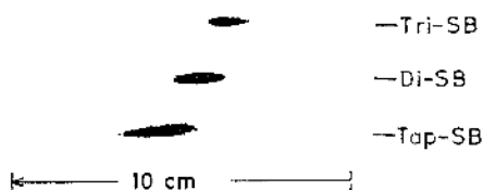
Figure 4. Chromatograms obtained by adsorption mechanism for reference SB-samples of tapered, diblock, and triblock type.
