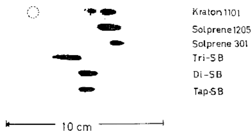
Figure 9. Chromatograms obtained by phase-separation mechanism for Kraton 1101 and others. A dotted circle indicates the final spot for the fastest component separated from Kraton 1101.
