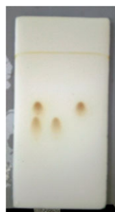
Figure 3. Photographs of chromatograms showing resolution of (RS)-Bisoprolol by use of BSA as chiral additive in stationary phase. From left to right: Spot 1: lower spot for ( R )-enantiomer and the upper spot for ( S )-enantiomer resolved from the racemate; Spot 2: pure ( R )-isomer and Spot 3: pure ( S )-isomer (both were isolated and characterized during this experiment, as described in the text).
