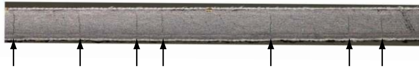
Figure 3: Transverse matrix cracks in a cross-ply laminate (after Sebaey et al. [67]).
