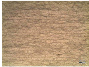
Spread-tow UD laminate (30 g/m 2 )
