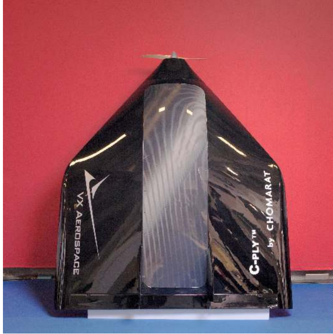
Figure 29: Excellent surface appearance of thin-ply non-crimp fabrics. Courtesy of Chomarats ©Laurent Becot Ruiz.
