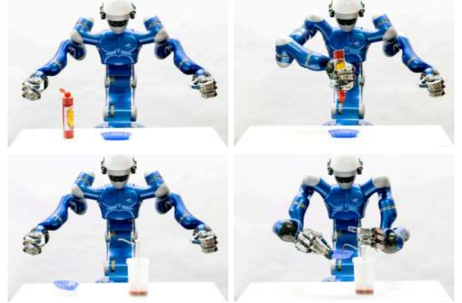
Fig. 6. The upper row illustrates serving ketchup by using a flexible plastic bottle, while the lower row shows the manipulation of a dispenser to achieve the same goal.
