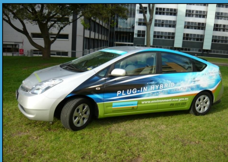
Figure 19: Vehicle-to-grid capable plug-in hybrid electric vehicle converted by UTS
