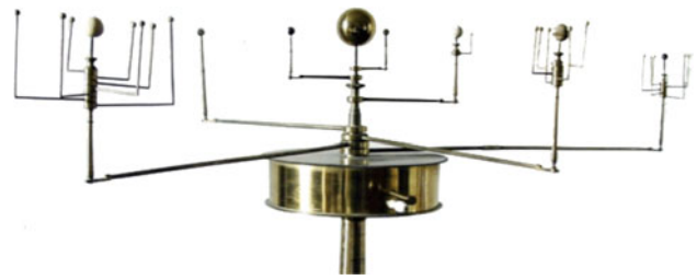
Fig. 11 In this mechanical orrery by Gilkerson, housed in the Armagh Observatory, the movement of the planets and their moons are mechanically simulated. It is not possible to access an arbitrary position of the system without moving through intermediate states. This is a feature of simulation systems: they do not have a closed form or analytic solution. To compute the state of the system at t_{12} , one must determine the state at t_{11} and move from there
