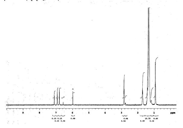
$^1\text{H-NMR}$  spectrum of H(CH<sub>2</sub>CH<sub>2</sub>)<sub>n</sub>(C<sub>4</sub>H<sub>3</sub>S) produced at 80°C in neat thiophene at 7.5 bar ethene pressure. (C<sub>2</sub>D<sub>2</sub>Cl<sub>4</sub>, 95°C)
