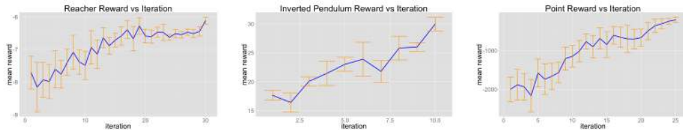
Figure 3: Reward vs training iteration for reacher, inverted pendulum, and point environments. The learning curves are averaged over 5 trials with error bars represent one standard deviation in the reward distribution at the given point.
