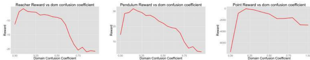
Figure 6: Reward of final trained policy vs domain confusion weight \lambda for reacher, inverted pendulum, and point environments.
