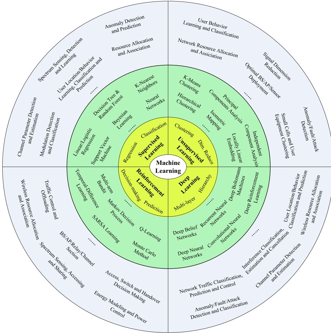
Fig. 4: The categories, characteristics and applications of ML algorithms.
