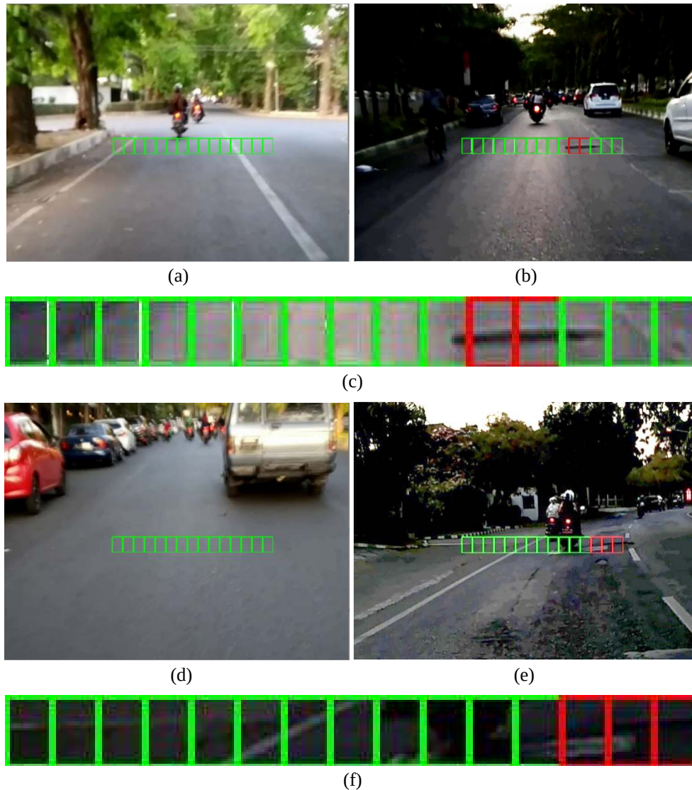
Figure 7. (a) & (d) are frames that do not have potholes in the road, (b) & (e) are frames that have potholes in the road and (c) & (f) are ROI that has detected pothole in the road
