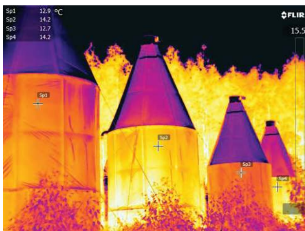
Figure 1. Infrared camera (FLIR) photograph showing control (orange) and elevated temperatures (yellow) in new experiments with the whole tree chambers at the Hawkesbury Institute for the Environment at the University of Western Sydney. (Photo J. Marshall.)
