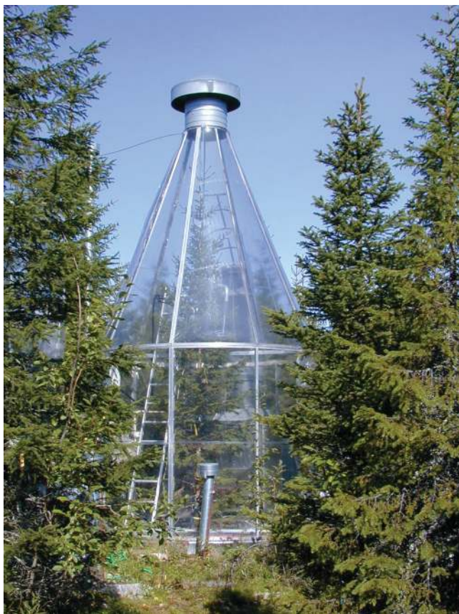
Figure 2. A whole-tree chamber enclosing a tree grown under ambient (poor) nutrient availability, ambient air temperature and ambient [\text{CO}_2] . (Photo S. Linder.)
