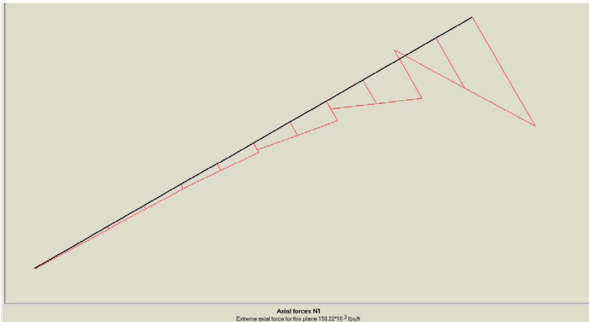
Figure 6.27. Axial forces in grouted zone for upper anchor after final excavation stage
