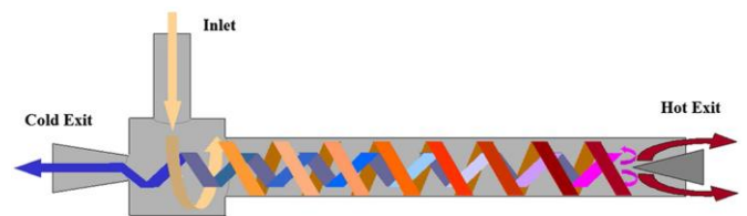
Figure 1. A schematic drawing of Ranque-Hilsch vortex tube
