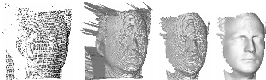
Figure 8. Pre-processing of the 3D scanner data, left to right: points cloud (sub-sampled 1:5); facial surface before processing; extracted facial contour; Beltrami smoothing result. Surfaces are rendered using Phong shading.
