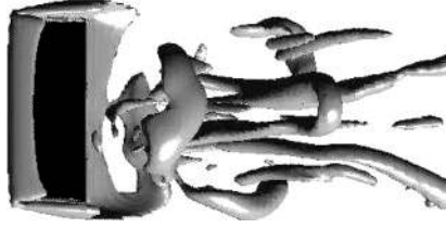
FIGURE 11. Top view of the asymmetric wake at large time behind a rectangular plate of AR=2 at \alpha=40^\circ and Re=500 . Vortices are highlighted with iso-contours of Q=2.5 . The flow is directed from left to right and the wing is shown in black.
