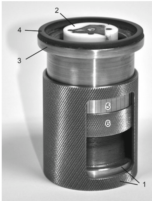
Fig. 5 Custom-made specimen holder for controlled manual grinding. The special grinding tool consists of two main parts. The inner part (1) secures the embedded specimen (2). The outer part (3) is equipped with an abrasion-resistant hard ceramic ring (4) which defines the grinding surface. An added scale (5) allows easy adjustment of a specific amount of abrasion and a look ring (6) ensures preservation of the setting during the grinding process
