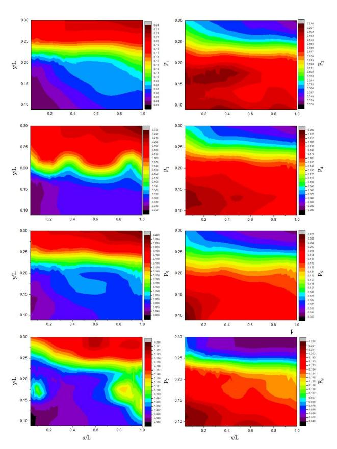
**Figure 9.** Contours maps of depth-averaged occurrence probability of octagonal bursting events (P<sub>1</sub>–P<sub>8</sub>) for the experimental run 4R.
