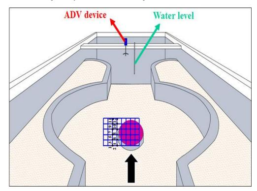
**Figure 1.** Overview of the laboratory flume employed in the present experimental study, with detailed views of the ADV device, the emerging bar (purple ellipse), and the measuring grid (in blue) composed of  $10 \text{ cm} \times 10 \text{ cm}$  cells. The black arrow denotes the flow direction. The measuring points analyzed are indicated listed from 1 to 12.
