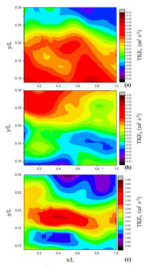
**Figure 3.** Contour maps of depth-averaged (**a**)  $\text{TKE}_x$ , (**b**)  $\text{TKE}_y$ , and (**c**)  $\text{TKE}_z$  for the experimental run 1R (no sand bar emerging from the flume bed).
