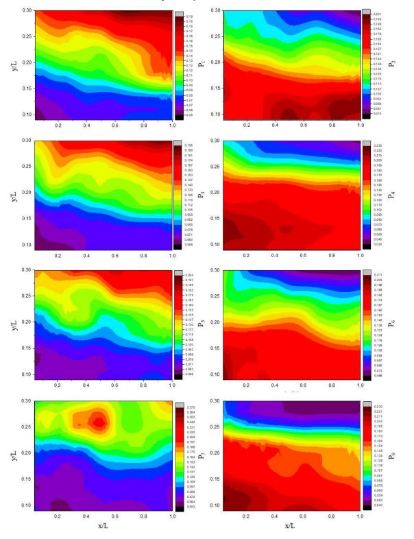
**Figure 8.** Contours maps of depth-averaged occurrence probability of octagonal bursting events  $(P_1-P_8)$  for the experimental run 2R.
