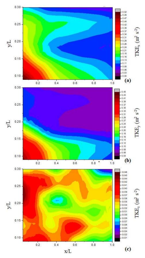
**Figure 7.** Contour maps of depth-averaged (**a**)  $\text{TKE}_x$ , (**b**)  $\text{TKE}_y$ , and (**c**)  $\text{TKE}_z$  for the experimental run 10R.
