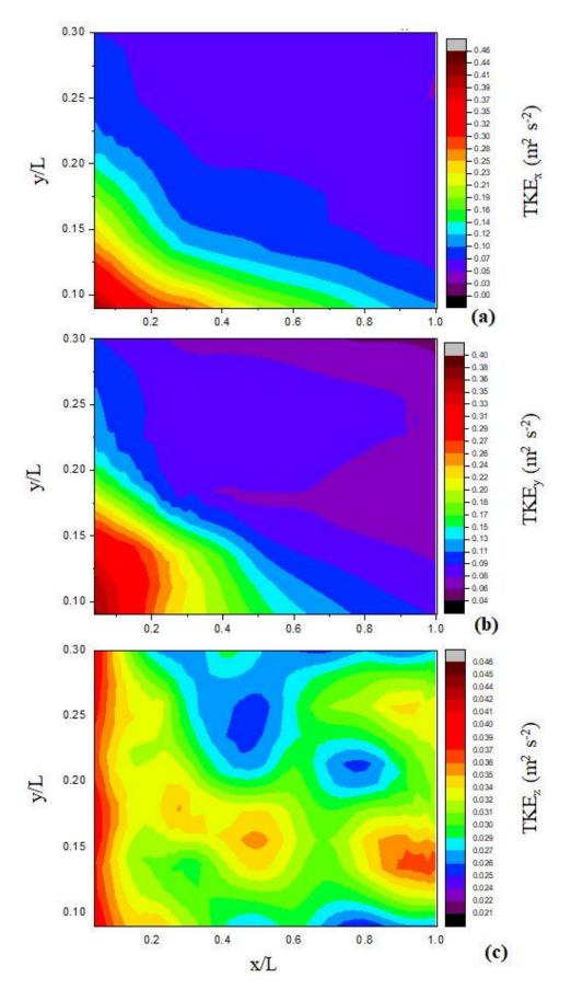
**Figure 6.** Contour maps of depth-averaged (**a**)  $\text{TKE}_x$ , (**b**)  $\text{TKE}_y$ , and (**c**)  $\text{TKE}_z$  for the experimental run 6R.
