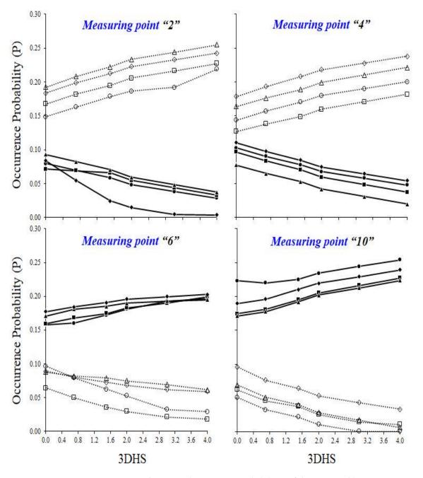
**Figure 15.** Depth-averaged occurrence probabilities of the octagonal bursting events with 3DHS values for the experimental run 10R:  $P_1$  (filled circles),  $P_2$  (unfilled circles),  $P_3$  (filled squares),  $P_4$  (unfilled squares),  $P_5$  (filled triangles),  $P_6$  (unfilled triangles),  $P_7$  (filled diamonds), and  $P_8$  (unfilled diamonds). Continuous lines indicate odd octagonal events, while dashed lines denote even events.
