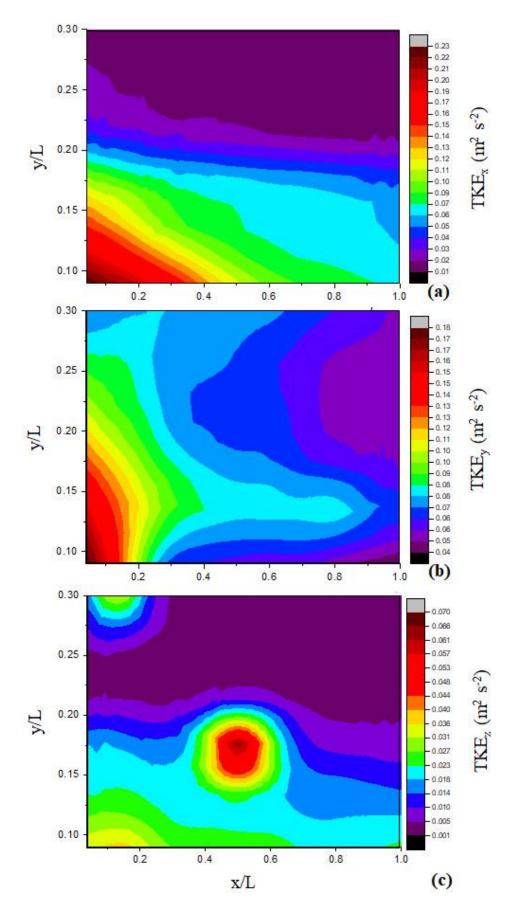
**Figure 4.** Contour maps of depth-averaged (**a**)  $\text{TKE}_x$ , (**b**)  $\text{TKE}_y$ , and (**c**)  $\text{TKE}_z$  for the experimental run 2R.
