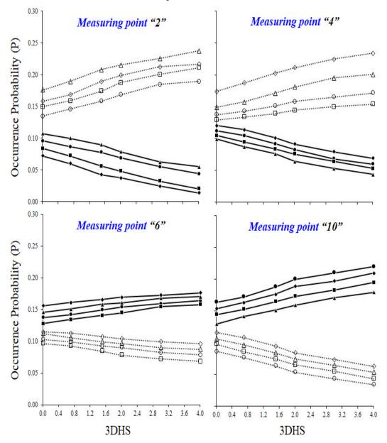
**Figure 12.** Depth-averaged occurrence probabilities of the octagonal bursting events with 3DHS values for the experimental run 2R:  $P_1$  (filled circles),  $P_2$  (unfilled circles),  $P_3$  (filled squares),  $P_4$  (unfilled squares),  $P_5$  (filled triangles),  $P_6$  (unfilled triangles),  $P_7$  (filled diamonds), and  $P_8$  (unfilled diamonds). Continuous lines indicate odd octagonal events, while dashed lines denote even events.
