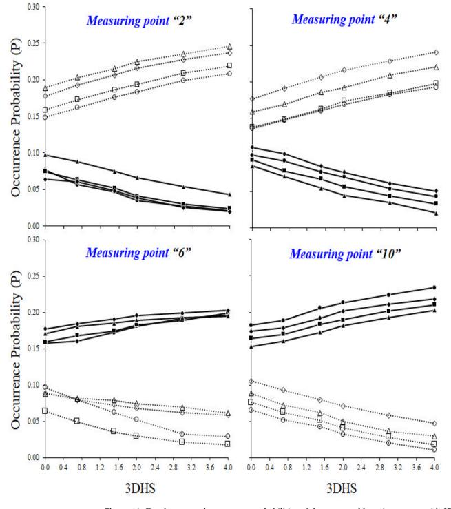
**Figure 14**. Depth-averaged occurrence probabilities of the octagonal bursting events with 3DHS values for the experimental run 6R:  $P_1$  (filled circles),  $P_2$  (unfilled circles),  $P_3$  (filled squares),  $P_4$  (unfilled squares),  $P_5$  (filled triangles),  $P_6$  (unfilled triangles),  $P_7$  (filled diamonds), and  $P_8$  (unfilled diamonds). Continuous lines indicate odd octagonal events, while dashed lines denote even events.
