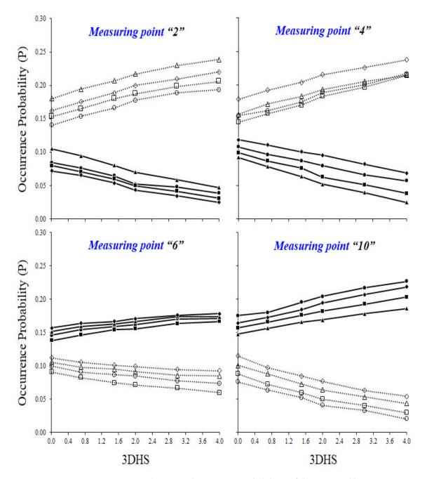
**Figure 13.** Depth-averaged occurrence probabilities of the octagonal bursting events with 3DHS values for the experimental run 4R:  $P_1$  (filled circles),  $P_2$  (unfilled circles),  $P_3$  (filled squares),  $P_4$  (unfilled squares),  $P_5$  (filled triangles),  $P_6$  (unfilled triangles),  $P_7$  (filled diamonds), and  $P_8$  (unfilled diamonds). Continuous lines indicate odd octagonal events, while dashed lines denote even events.
