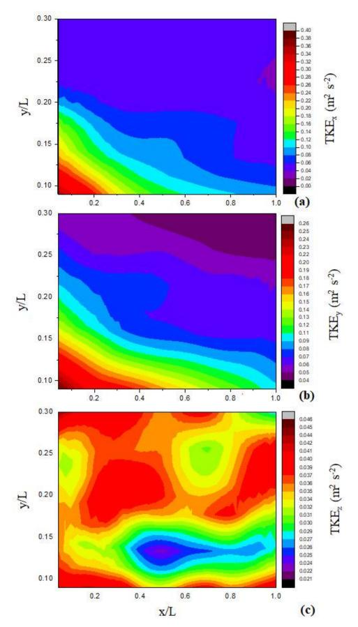
**Figure 5.** Contour maps of depth-averaged (**a**)  $TKE_x$ , (**b**)  $TKE_y$ , and (**c**)  $TKE_z$  for the experimental run 4R.
