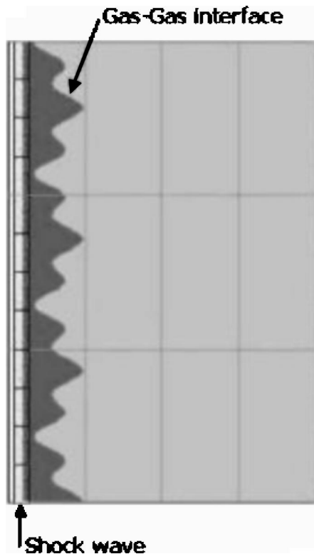
Fig. 16 Richtmyer-Meshkov instability simulation, time t = 1.3\tau_m where \tau_m is the Argon-Argon mean collision time. The shock wave is ahead of the gas-gas interface.
