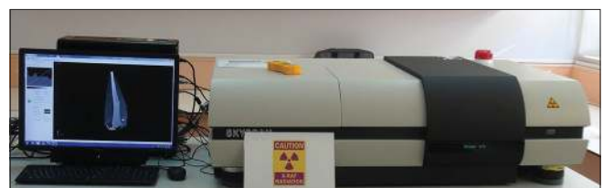
Figure 3: Micro-computed tomography for analysis of mineralized tissues with micro-sized sections
