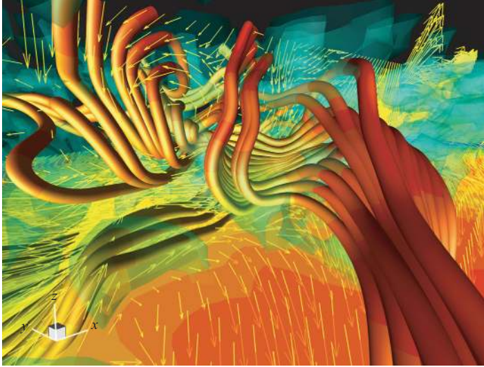
FIGURE 12. Instantaneous flow structure of the incoming boundary layer: upper region ( z/\delta = 0.6\text{--}1.0 ). Semitransparent vorticity magnitude isosurfaces for |\omega|\delta/U_\infty = 0.5 are shown. Velocity vectors with a convective velocity of 0.8U_\infty are shown in two planes; at y/\delta = 0.5 and z/\delta = 0.6 , the latter flooded with streamwise velocity contours. Streamlines are computed within this convective reference frame.
