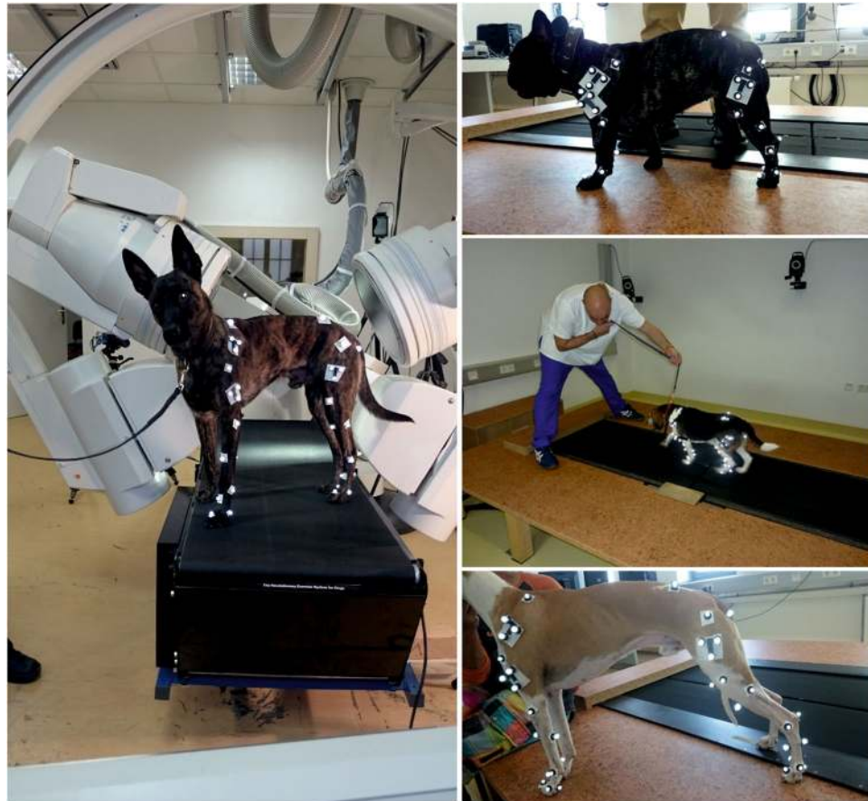
Figure 10. Jena X-ray Lab (left) and locomotion lab Hannover (right). All four breeds were measured in both labs. Marker were set under fluoroscopic control. Fluoroscopic data was used for Scientific Rotoscoping. Marker-based 3D kinematics were recorded at the locomotion lab in Hannover.
