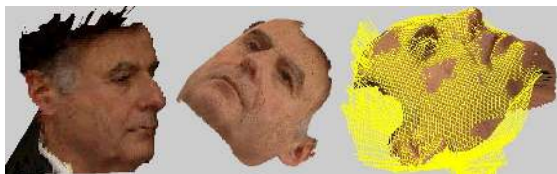
Figure 7: Matching results after fine alignment. From left to right, the 2.5D test scan, the 3D model, the 3D textured model overlaid by the wire-frame of the test scan after fine alignment.
