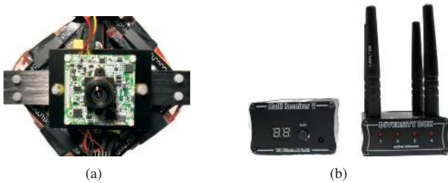
Fig. 15. The UAV vision system: (a) CTDM-5351 camera installed on board, in the lower part of the quad-rotorcraft; (b) 4-Antenna Diversity System Receiver connected to the ground station PC.
