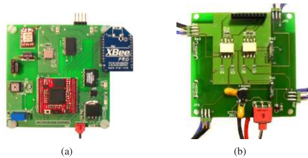
Fig. 12. The electronics on board: (a) Electronic card for the DSP, analog rate gyros, IMU connections and wireless modem; (b) Signal conditioning board.
