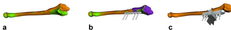
Fig. 1 Preoperative Plan. Outline of the investigated computer-assisted planning approach. a Quantification of the malunion by superimposing the proximal part of the pathological bone (orange) with the mirrored contralateral bone (green). b Simulated reduction of the distal fragment (violet) and positioning of the fixation plate. The (beige) cylinders represent the angular-stable locking screws. c The screw models are transformed back to the pathological bone by applying the inverse transformation. The patient-specific drill and cutting guide (beige) is designed based on this information
