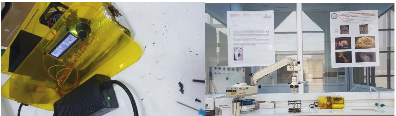
Figure 3. Extrusion device and HA-PLA filament preparation.
