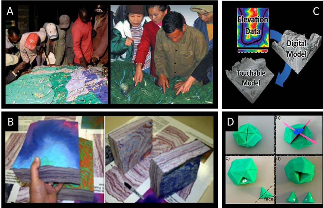
Figure 6. Examples of 3D printing applications in education and communication. (A) Ghawana and Zlatanova (2013) review 3D printing applications for urban planning, with public participation in planning using a 3D printed terrain model shown. (B) shows a 3D printed seismic volume as a way to visually enhance spatial perspective (Reyes et al., 2008). (C) Hasiuk and Harding (2016) discuss the use of 3D printing digital terrain models for use in teaching. Shown is an example workflow for printing the Grand Canyon. (D) Casas and Estop (2015) used 3D printed dissection models for teaching crystallographic concepts.
