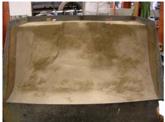
(c) test 3, non soil nailed no curvature slope
