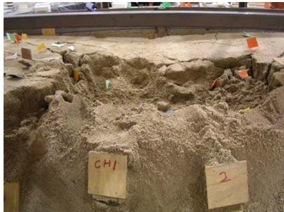
(a) test 1, soil nailed convex slope
