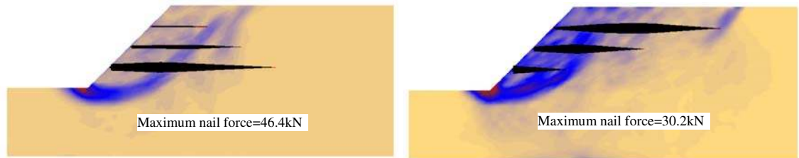
(a) short nail at top, FOS=1.34 (b) short nail at bottom, FOS=1.22
